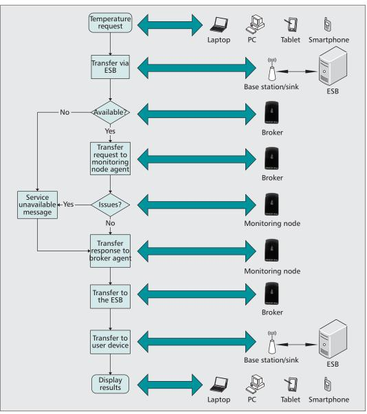
A novel feature of our system is that it makes possible offering services that are retrieved not by actual nodes with actual sensors, but as a result of a data aggregation process, in a way so similar for any human user of our system that we refer to it as sensor virtualization.
