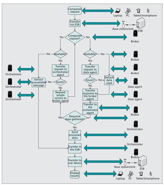
Figure 4. Composed service request processing.
